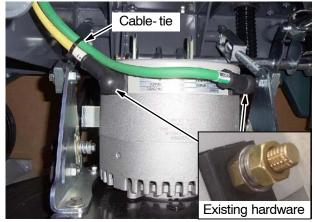
2. Using the hardware supplied with kit, connect the cables to motor as shown. Make sure to position the cables at the angles shown. Torque the nuts to 100 in-lbs (11.3 N-m).
